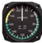
Dual Scale (MPH/Knots) with multicolor markings
