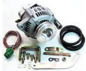
The AL12-EI70 kit includes a high output AIRCRAFT alternator with an exclusive internal crowbar over-voltage protection circuit. The alternator is fully pilot controllable through unique internal wring. The dual internal fans are designed for aircraft engine rotation for maximum cooling. The AL12-EI70 kit includes the tension arm, mounting brackets, all required AN hardware, and V-Belt for Superior and most Lycoming engines with a 9-3/4 engine pulley.
