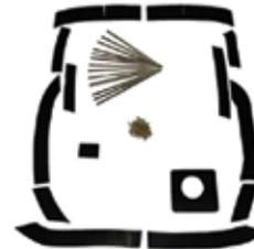
FAA-PMA Approved Baffle Seals for 172R/S Cessna Aircraft.
