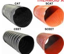
"CAT" - "CAT" type flexible hot or cold air ducting is extremely lightweight and highly flexible. Short lengths can be joined together to form a continuous length. Made of a single ply black neopreneimpregnated fiberglass with a spiral copper coated steel wire inside and wrapped with fiberglass cord on the outside. Suitable for conveying fumes and air a temperatures from -65° to over 350°F. Not recommended for handling liquids or highly abrasive materials, or for negative pressure applications.
