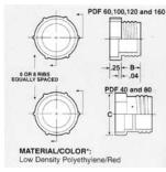
Series PDF plugs are designed for easy mechanical or hand installation on flat-faced O-ring fittings.
