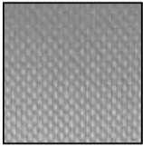
1.45 oz./sq. yd. Lightweight Industrial Cloth used in Osprey and other designs. Widely used by model builders, known as "Deck Cloth", Thread Count 60 x 47.
