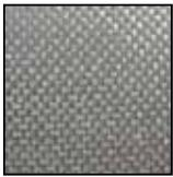
3.74 oz./sq. yd. Light weight Boat or Tooling Cloth. Tight plain weave. Thread Count 24 x 22. Breaking Strength. 160 x 135 lb./in. Finished Weight 3.60 oz./sq. yd. Thickness .0055"
