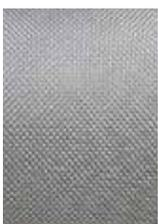
Knitted fabrics are a relatively new format in composites. The performance of the glass is greatly enhanced by removing the interstices of the woven fabric and the crimped condition. E-glass in woven goods normally has 22,000 PSI tensile strength. Layered nonwoven goods give 27,000 PSI which is about a 20% improvement. Knitted glass offers greater ease of fabric orientation and saves time over multi-layered wet lay-ups.
