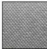
9.66 oz./sq. yd. Heavy Weight Boat or Tooling Cloth. Plain Weave. Thread Count 16 x 14. Breaking Strength 450 x 410 lb./in. Finished Weight 9.40 oz./sq. yd. Thickness .014".
