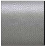
3.16 oz./sq. yd. Lightweight Industrial Cloth with aerospace applications. Excellent for model building. Only .004" thick. Crowfoot weave, which contours nicely. Thread Count 60 x 58. Breaking Strength 125 x 120 lb./in. Finished Weight 3.08 oz./sq. yd.
