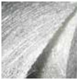
100% Fiberglass in a non-woven state. It is used for bulk "build-up" in molding and fabricating components. Also useful for filling holes and badly damaged parts. 1.5 oz. Weight. 38" Width.
