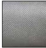
8.5 oz./sq. yd. Lightweight boat or tooling cloth. Threads per inch: 18L x 18W. Used in Osprey aircraft and other homebuilts.
