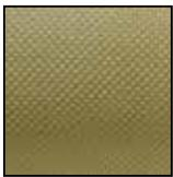
5.79 oz./sq. yd. Lightweight Boat Cloth. Flat weave, not twisted. Thread Count 18 x 18. Breaking Strength 250 x 225 lb./in. Finished Weight 5.85 oz./sq. yd. Thickness .010".
