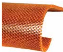
AHN 7800 is an Commercial Grade Nomex honeycomb particularly suited for use where resistance to corrosive attack and moisture are important. This material exhibits good strength characteristics and is fire resistant. It is available in a variety of cell sizes and densities to suit most purposes. Typical applications include light-
