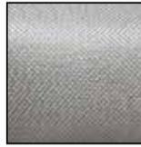
5.85 oz./sq. yd. Lightweight Boat or Tooling Cloth. Plain Weave. Thread Count 18 x 18. Breaking Strength 250 x 250 lb./in. Finished Weight 5.64 oz./sq. yd. Thickness .009" as used on KR Aircraft.
