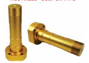
500X5 AXLE - Machined from 2024T3 aluminum. Gold anodized per specification MIL-A-8625C, Type II for improved corrosion resistance. Length 5-3/4". Mounting bolt pattern is four equally spaced 1/4" dia. holes on 1-15/16" dia. bolt circle. Thread size: 1-1/4 x 16.
