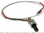
P-Leads are a critical part of the ignition system and their good condition is vital to safety and airworthiness. P-leads are often overlooked and seldom replaced because replacement p-leads are not available from the aircraft manufacturer and materials to fabricate new p-leads are not commonly available. Because most leads are shielded, mechanics do not
