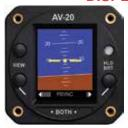
Complement Your Panel with a Certified (NORSEE) 12-In-1 Display that adds a suite of in-flight information to nearly any panel. Designed to seamlessly fit in a standard 2 1/4-inch round instrument opening, the AV-20-S offers a standby attitude indicator, angle of attack, bus voltage, slip/skid Indication, outside air temperature, density altitude, G meter, and more—all protected with a 30-minute internal battery backup for uninterrupted function in the event of power
