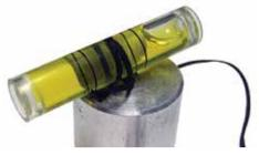
This extremely simple and sensitive tool uses the plum-bob and bevel rnis extremely simple and sensitive tool uses the plum-boo and bevel principle to balance props both vertically and horizontally. It can be carried in a small tool box for easy use in the field and balances props accurately for smooth operation. The precision machined hub works with any prop designed with standard 1" center hole. Illustrated instructions included ... .....P/N 13-17400
