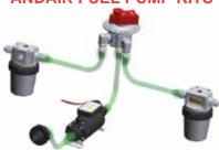
These systems have a PX375-TC Fuel Boost Pump either for 3/8" or 1/2" fuel lines and GAS375 Gascolator, Some kits may have two Gascolators: one with the standard flow direction (Right to Left) and one with the reverse flow (Left to Right), mounted in the wing roots.
