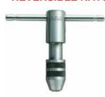
General's Reversible Tap Wrenches feature a fine-tooth ratcheting mechanism which adjusts on the fly for right - and left-hand use. In addition, the ratchet can be locked to transform the tool into a standard tap wrench. The self-centering, hardened-steel jaws assure the formation of straight threads in your work piece. Although designed mainly for holding taps, the Reversible Tap Wrench also works great with reamers, drill bits, screw extractors and other hand-turned tools.
