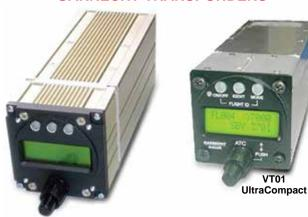
The Garrecht Transponder VT-01 is a flexible and modular system concept, in a compact size (57mm) with a very low current and integral alticoder. Available as Class-1 (125 Watt) or Class-2 (71 Watt) System. Specifications: Certification i.a.w: ETSO-2C112a, ED-73B
