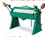
Tennsmith's heavy duty universal hand brake is a great tool for a wide range of sheet metal binding and forming operations in 12 gauge and lighter mild steel. The brake is ideal for both box and pan and straight bending in hold and cold rolled plate, stainless steel, aluminum, and heavy plastic. Welded steel plate construction for strength
