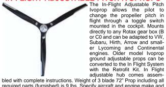
The In-Flight Adjustable Pitch Ivoprop allows the pilot to change the propeller pitch in flight through a toggle switch mounted in the cockpit. Mounts directly to any Rotax gear box (B or C0 and can be adapted to VW, Subaru, Hirth, Arrow and small-
