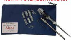
This 3 Stone Rotary Cylinder Kit makes available an effective tool to recondition the interior running surface of the oleo cylinder barrel, and is intended to be used each time the MLG oleo struts are disassembled for routine seal replacement or when upgrading to the popular Main Landing Gear Oleo Restoration Kit (STC SA01247CH).
