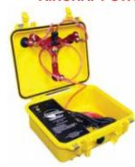
SA3Y-P-UNI-2 Aircraft Static Test Adapter. • Automatically attaches to aircraft fuselage • High pressure hoses with quick release fittings • Press to release button for static adapter removal · Safety check valves for power failure and system leaks · High impact yellow case with internal electric vacuum pump · Designed to fit most general & military aircraft static ports
