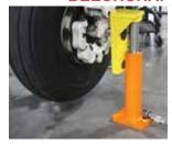
The pad is available without the remote bottle jack. The 30M-B90 Jack Pad is bottle jack. The SUNN-BBU Jack Fau is great for raising one wheel for a tire change, repacking wheel bearings or servicing the brakes. When used with a long stroke jack, the jack pad may be used to change a flat tire. Small and light enough to carry on board, the jack pad adds mission capability when operating from airports that do not have full service or wing jacks large enough to lift these aircraft
