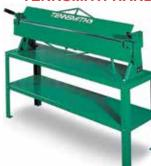
Versatile, economical hand brake designed for straight forming of mild steel in thicknesses of 22 gauge & lighter. Made in the U.S.A by Tennsmith. Bends material up to 48" wide. Wts: brake: 280 lbs. Optional stand: 95 lbs. Ideal for bending materials used in light aircraft construction. Shipped direct to you from factory in Tennessee.
