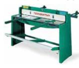
Tennsmith squaring shears offer precision shearing and rugged construction. These shears feature traction, ground alloy tool steel blades to prevent material movement during shearing. Will shear material up to 16 gauge mild steel and up to 20 gauge stainless steel. Both blades are adjustable and back gauge gives highly accurate readings. Wts: Model 36: 700 lbs.
