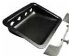
4 HOLE RECESSED MIC & PHONE JACK HOUSINGS - Modified to allow plugs to enter from the opposite side, being recessed they are out of the way. When jacks are plugged in they are flush with the edge of the housing. Made of aluminum, with a powder coat finish. Comes bagged with housing, clamp, mounting screw. Dims: 4"W x 5"L x 1.06"H; Cutout req.: 3.25"W x 4.43"L
