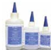
Polyfix™ 14000 Thin Cyanoacrylate has a super thin viscosity that penetrate deep into cracks by capillary action and cures in a matter of a few seconds. Surfaces to be bonded must be tight fitting and should be held together while you apply the ca around the edges of the seams at the moment ca's cure they give off a vapor that can irritate the nose and eyes, so be prepared. Thin ca's work very well
