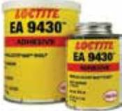
Replaces the EA-9410-2 glue. EA-9430 has the same characteristics as the EA-9410, but has a 50 minute pot life instead of the 30 minute pot life of the EA-9410 at 77°F. Used extensively in the Strojnik S2A sailplane and many other homebuilts.
