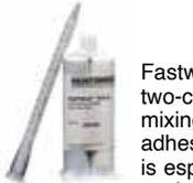
Fastweld 10 A/B epoxy adhesive is a rapid-setting, two-component paste offering a convenient one-to-one mixing ratio by volume or weight. Fastweld 10 A/B epoxy adhesive produces strong bonds in a very short period. It is especially suited for bonding small parts and for repair work. Pot life: 3-4 minutes at 77° F, Cure Time: 4 hours.
