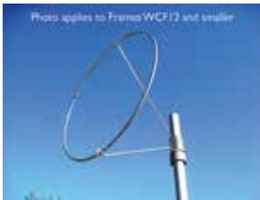
Small Frames (12" and smaller) - Lightweight frames made of galvanized steel wire. Large Frames (18" and larger) - These are heavy duty frames designed to withstand storm force winds and harsh environmental conditions. Large frames are made of galvanized steel (WCF18) or a combination of steel and cast aluminum (WCF20, WCF22, WCF24).
