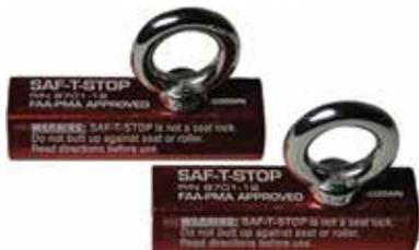
Saf-T-Stop is an auxiliary seat stop mechanism approved by the FAA for use with Cessna seat track A.D. #87-20-03. Installs easily, sliding over seat track. Approved for: Cessna 150, 152, 170, 170B, 172, R172, 175, 180, 182, 185, 190, 205, 206, 207, 210, 303, 337. Not a seat lock, Saf-T-Stop is designed to restrict rearward motion if the seat lock fails.
