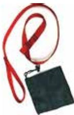
Pocket tow makes tail wheel aircraft maneuvering easy. Made with one-inch heavy-duty nylon webbing, the lightweight tow bar alternative is small enough to fit in your pocket and works on tail wheel aircraft with a 360-degree full-swivel tail wheel assemblies. The small end loops around the tail wheel leaf spring and cinches up tightly to pull and steer the aircraft backwards without pushing or pulling on any flight surfaces.
