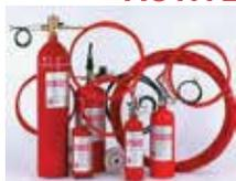
Active Extinguishing Line is totally independent, 1kg, fire extinguishing system from any power source. Its main secret lies in the heat detector in a form of a line made out of special laser predriller polymer, which will react instantly to any source of heat or fire. This line (heat detector) is connected to reservoir containing fire-extinguishing agent: hexafluoropropane
