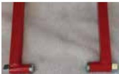
Beech Adapter. With this adapter you can move Beech Aircraft with the little tow pin. This adapter fits any towbar with a 3/4" or larger hole. Note: The grip length; (distance from nut to bolt head) is 1 1/2". With this adapter you can move Beech series aircraft with the small pin.
