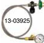
**TR-55 00GSE-1008-00** Standard length 18 inches. The TR-55 is the most economical way to fill your cylinder. One side has a CGA-540 nut & nipple with an O-ring seal, while the other end is equipped with a large hand nut with bare nipple. This allows you to slowly and safely bleed the line so the fittings can be easily removed from the cylinder.
