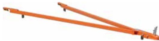
Lightweight aluminum designed for Waco, Stearman, & Cessna 195 type aircraft. Length: 100", Spread: 90", Wt: 22 lbs. Hook dia: TR-71 (.850), TR-72 (1.25). TR-71R Towbar w/Ring hitch.
