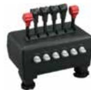
TWIN ENGINE. Fully programmable and featuring six physical detent axis' and up to 350 buttons. Throttle Quadrant USB takes you from the computer to the cockpit. **Features:** 6 Axis 12 Buttons (24 Button functions w/Control Manager Software included), 6 Physical Detents, Fully Programmable with CH Control manager, Compatible with Windows 98, Windows ME, Windows 2000 & Windows XP. Compatible with all Windows based Games.....P/N 13-03377 .....**\$132.75**
