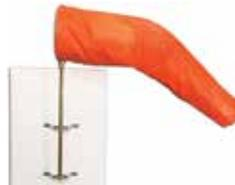
These complete USA made windsock kits include our aviation quality orange windsock, standard aluminum frame, heavy duty windsock ties, 30" long galvanized pole with 3/4" pipe thread, and mounting brackets. They are a stand alone unit for mounting on a flat vertical surface. Windsock size 18" diameter by 48" long ..... P/N 13-24023 ..... \$121.80
