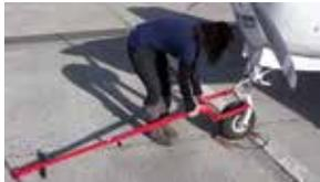
The 04M-BBU is unique because it can attach to virtually any aircraft. It has interchangeable "Feet" that can be matched to any aircraft. Each of the "Feet" typically adapts to several models or series of aircraft and several sizes can be carried right on the tow bar. This is perfect for FBO's that deal with a variety of aircraft or aircraft owners that have more than one plane or shared hangars. "Interchangeable feet sold separately".
