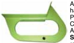
Airforms P/N AF2612035-1, Tail tie down handle, rear. Direct replacement for Cessna P/N 2612035-1. Eligible for all S/N aircraft, Cessna models 208 and 208B. FAA PMA Approved.
