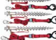
Big-Screw EZ Tie-Down is an innovative tie down system combining a lightweight 18" cast aluminum ground screw, and a custom aviation designed attachment strap. The 18-inch long cast aluminum screw provides stronger ground holding in all soil types. The screw penetrates deeply into compacted soils resulting in superior holding strength.
