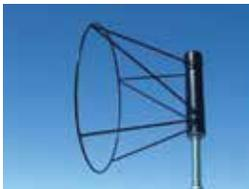
The ball bearing windsock frames are a rugged design constructed of a welded steel construction and then a powder coated finish for corrosion protection. They incorporate a two bearing pivoting design for effortless pivoting. These frames are ready to be mounted on a 3/4" female pipe thread for the 8", 13", 18" and 24" and a 1" pipe thread for the 36".
