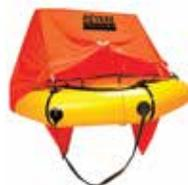
Double 200 lb. SuperRev™ ballast pockets, it enhances stability in rough sea conditions. Its light weight allows for easy deployment and the compact size makes stowage easy in the smallest of spaces. Operation is easy. Just open the red flap on the valise and extend the painterline. Give a hard pull and the raft inflates automatically in less than 30 seconds. Coastal Compact Raft is not recommended for offshore use.
