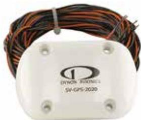
The SV-GPS-2020 GPS Receiver/Antenna from Dynon Avionics allows existing and SkyView and Advanced AF-5000 series customers to add a 2020-compliant GPS position for ADS-B Out. As a drop-in replacement for the existing SVGPS-250 receiver, existing customers do not need to run any additional wires, coax, or install any new boxes in their aircraft. When combined with Dynon's SV-XPNDR-261 Mode-S transponder,
