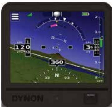
D3 lets pilots supplement their unreliable legacy instrumentation with an affordable, portable electronic attitude indicator that works. The D3 features the same reliable, proven AHRS engine from Dynon's best-selling panel-mounted products for experimental, light sport, and type certificated aircraft.
