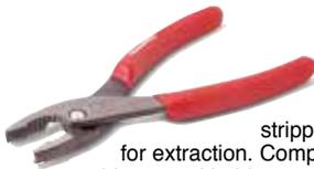
These Slip Joint VamPLIERS have the signature concave shaped jaws with vertical and horizontal serrations designed inside of the jaws. This which gives the perfect bite around a stripped/rusted/corroded screw, nut or bolt for extraction. Compared to its predecessor, these jaws are wider to tackle bigger problem screws. Adding to its big bite is the "slip-joint" feature made with reversed body structures that allows the jaws to adjust and firmly take on bigger screws, nuts, and bolts!
