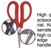
High quality scissors for cutting Kevlar thread. These scissors are specially designed for cutting Kevlar material; Kevlar thread in particular. One blade is micro-serrated along the whole edge. The blades are made of high carbon alloy steel with Molybdenum and Vanadium edge 60~62, cutting edge hardness HV1200. The handles are especially designed for firm grip and to ease repetitive cutting action.....
