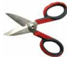
The VT-3949 Eshears are made of high carbon stainless steel with Molybdenum and Vanadium blades, vacuum hardened and precision-ground for a long lasting edge. These sport modern ergonomic handles that are made of Nylon with 30% fiberglass and work for both the right and left handed user.
