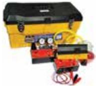
This small test kit is designed to allow the aircraft mechanic a convenient and economical way to purchase the basic small engine test equipment. This kit contains: 1 - TP104 Cylinder Pressure Tester, 1 - TP105 Magneto Timing Light, 1 - TP102 Timing Indicator, 1 - TP103 High Voltage Cable Tester, 1 - TP216 Tool Box
