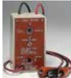
Gives a fast, accurate test of high voltage aircraft ignition cables. Simply connect 3 wires, push test button and test is completed. The E5 will instantly indicate in its test window both good and defective cables - no waiting for indication to appear. Fail-safe circuitry. Heavy-duty lead wires. Compact 3" x 5" x 2-5/8" case. Wt. 1-1/2 lbs. .... P/N 12-01016 ..... **\$109.75**
