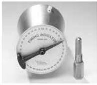
The Aircraft Timing Indicator Model E25 is a unique device that locates the relative relationships between the crankshaft, magneto point openings, camshaft and valve timing. Easily attached to the propeller spinner with mounting bands that are included with the unit, the E25 quickly and accurately (within 1/2 degree!) locates top dead center. The result: the all-aluminum
