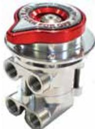
SPRL V9-4 duplex valve with ceramic disc valves for feed and return. It is tapped 1/4" nps feed and return and will take standard npt fittings and our -6 banjos.
