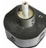
These premium fuel valves are recommended by Rutan Aircraft as the best fuel valves they have seen. They are a direct, bolt-in replacement for Weatherhead and other fuel valves. They turn smoothly and freely with a very positive spring loaded ball detent system which lets you feel the left right and off positions. Manufactured of anodized aluminum.
