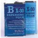
This system consists of two components - "X-30" Resin and "X-30" Catalyst. When the resin and catalyst are mixed in equal volumes they expand into a rigid closed-cell foam of 2 pound density. Thorough mixing of the two components is essential. "X-30" Foam expands approximately 40 times its liquid volume.
