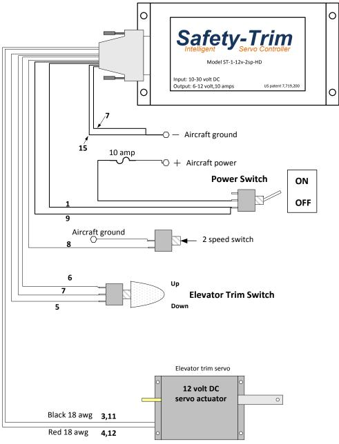
NOTE: Parallel connections of power, ground and servo wires are for applications with servos rated at more than 5 amps
