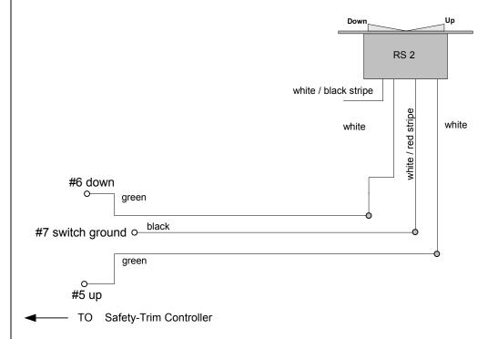
Note: RAY ALLEN Rocker Switch RS2 is of a custom design, in the neutral position the white wires are shorted together
