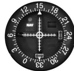
Figure 5: Analog OBS indicator set to 150
