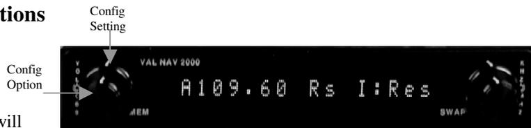
Figure 3: NAV 2000 in Configuration Mode
