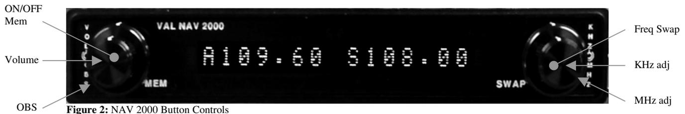
Figure 2: NAV 2000 Button Controls
