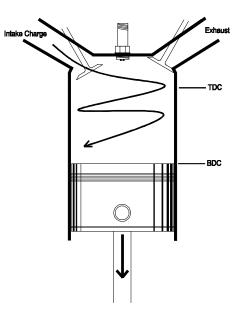
Fig. 3: Shows the swirling pattern of the fuel/air charge during the intake stroke.
