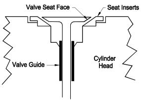
Fig. 8: Shows an exhaust valve, seat and guide.
