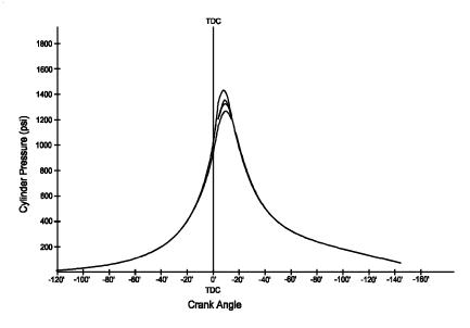
Fig. 2: Typical cycle-to-cycle variation when operating on the lean side of peak EGT (LOP).
