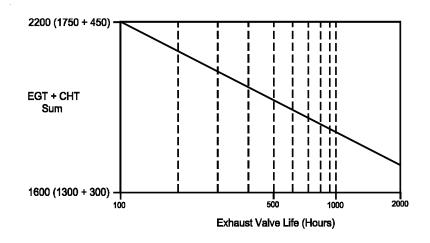
Fig. 9: Shows the affects of heat on the life of an exhaust valve.
