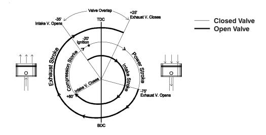
Fig. 7: Typical valve timing diagram.
