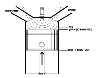
Fig. 4: Shows the position of the piston (20í before TDC) when the spark plug is ignited.
