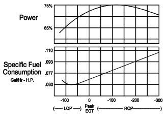
Fig. 6: Typical power curve and specific fuel consumption for most aircraft engines.
