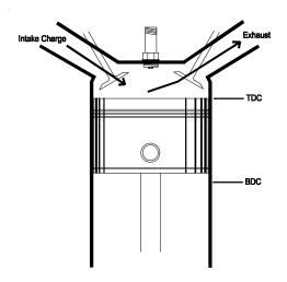
Fig. 1: Shows the exhaust exiting the cylinder at the end of the exhaust stroke and during the start of the intake stroke. direction). As the intake valve opens (approximately 35 degrees before the piston reaches top-dead-center "TDC"), the exiting exhaust gasses continue to flow out the exhaust port. This helps to keep the pressure in the combustion chamber low so the intake charge can be drawn into the cylinder as the exhaust gasses continue to vacate (see Fig. 1).
