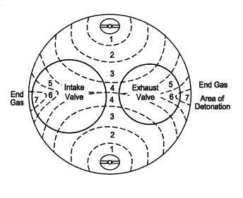
Fig. 11: Burn pattern for a Continental O470 combustion chamber.
