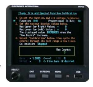
**"Powered By":** The control pot can be powered by the aircraft bus (preferred) or the by the EDC. If the control pot is powered by the aircraft bus, the MVP must do a ratio metric calculation to insure the flap readings do not change when the bus voltage changes.
