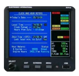
The "#Cycles" can be setup to count airframe (takeoff/landing) cycles or engine start cycles. The value of "#Cycles" is based N1. When a preset high value of N1 is reached the "Status" field will display "Armed." Then, when a preset low value of N1 is reached the "Status" field will display nothing and the value of "#Cycles" will be incremented by one.
