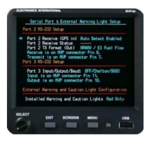
**"Port 2 Receive Status":** When the Port 2 Receive field is set to "Auto Detect Enabled" the Port 2 Receive Status field will show one of the following:
