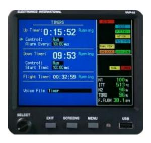
**'Flt Timer:**" The Flight Timer automatically times each flight. The Flight Timer is reset and started when the N1 exceeds 97%. The Flight Timer is stopped when the N1 drops below 60%. The start and stop N1 settings may be changed in the "Engine Data, Hour Meters and Flight Timer Setup" screen found in the "System Configuration Screens Menu. Only the installer (using the maintenance password) is authorized to make these changes.
