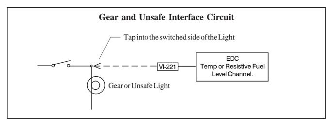
There are three options for interfacing the EDC to the aircraft's gear system.
