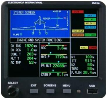
When the ailerons are trimmed the bar graph to the right of the display will move up or down from the horizontal line. The bar graph should move up as the right wing is trimmed up. Neutral is indicated by a single bar on the horizontal line.
