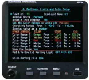
**"Set the Color Ranges in units of:"** The Color Ranges for a Function must be set in the units listed in this field. The "Display Units" field sets the units in which the Function will be displayed on the Main Engine Screen.
