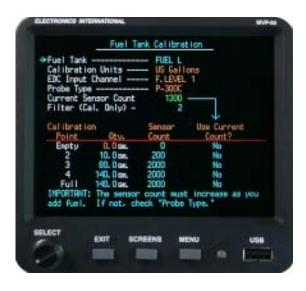
"Calibration Filter": When fuel is added to the tank the sensor count will increase. When you stop adding fuel to the tank the sensor count will continue to climb for a short period of time and then stop climbing. If the sensor count does not settle out (continues to jump up and down), increase the "Calibration Filter." The higher the Calibration Filter the more stable the counts will be and the longer it will take for the sensor counts to settle out.
