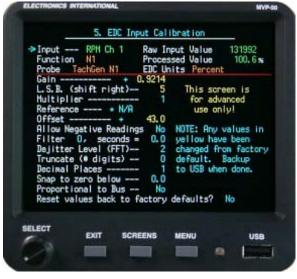
**"Filter:"** The Interim Value may be filtered. A filter increases the response time (shown in the "seconds =" field) and reduces jumping.
