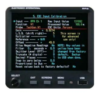
**"Probe:"** This field displays the Probe assigned to the EDC Input selected above.
