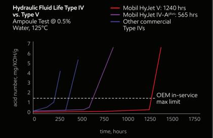
Side-by-side testing confirmed that Mobil HyJet V hydraulic fluid offers better stability and longer in-service life than Type IV fluids.
