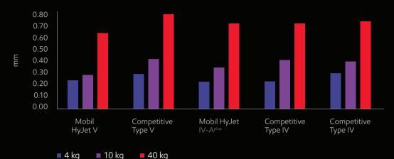
Wear Scar in mm after one hour at 600 rpm, 75°C and force as shown.
