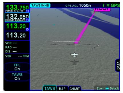
The status is displayed on a background indicating the severity of the condition; red for warnings, yellow for cautions, and cyan for
