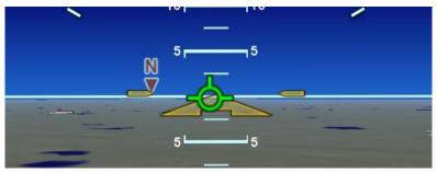
The Setup Page also provides a means to control whether the Horizontal Deviation Indicator (HDI) is always visible or shown only for approaches.
