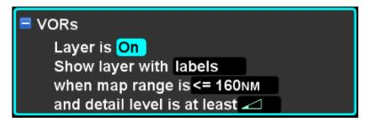
Like the airport filter, the layout and wording of conditions within a map layer is designed to make the set of conditions read like a sentence. The sentence is structured to clearly specify the set of conditions that must be met in order for items in the layer to be shown. Each of the possible criteria is described in the sections below.
