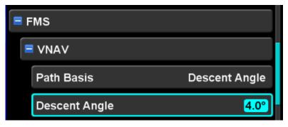
Using the enroute VNAV altitude target and the associated waypoint, the IFD will project that angle along the flight path all the way to the current aircraft altitude. That point is depicted on the map as a green circle labeled "TOD" (top-of-descent). When enroute VNAV is allowed and the aircraft reaches the TOD point, the IFD will automatically commence enroute VNAV.
