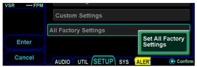
To apply the preset, press the right knob, the ENTR button, or the "Enter" LSK, or touch the green dialog. To abort the preset, press the CLR button or the "Cancel" LSK. Once a preset has been applied, the list of presets will be dismissed and the normal Setup Page contents will again be displayed.
