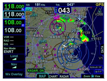
Onboard Weather Radar Overlay on Map
