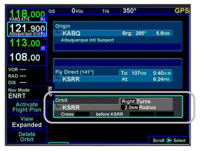
If the orbit radius is larger than the distance from the aircraft to the orbit fix, then the aircraft will intercept the orbit on the extended radial between the orbit fix and the aircraft. Just like a traditional holding pattern, there is no insert cursor between a fix and a subsequent orbit. The only way to get out of an orbit is to command a Direct-To or activate a different leg. The orbit size can be changed while it is active but no path to reacquire the orbit is depicted on the map.
