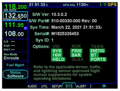
When the aircraft is not airborne, the Software Status Page will also show a "Download Logs" LSK. Pressing that LSK will put the IFD into Maintenance Mode where the datalogs can be downloaded (see page 7-68 for instructions).
