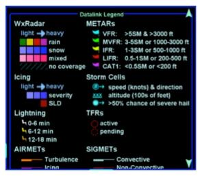
At large map ranges beyond 250nm from the aircraft, small areas of high-intensity radar returns may not be displayed; instead, larger areas of surrounding lower-intensity radar returns will be shown.
