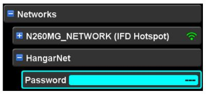
Editing the password for an external network is accomplished using the normal technique for a textual field. If no password has been entered, then the field will show three dashes. While the password is being edited, the characters will be shown. However, as a security measure, once the password has been accepted, the field will be shown as four asterisks.
