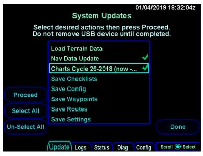
Once the set of items to be loaded has been selected, press the Proceed LSK to start the load.
