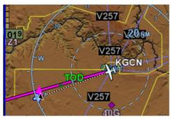
When a target vertical speed is specified, the IFD will compute the TOD point using current groundspeed and the desired descent rate. However, when the aircraft reaches the TOD point and enroute VNAV is allowed, the IFD will compute the angle required to reach the desired altitude, then commence with enroute VNAV using that angle.
