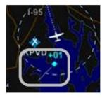
Since TIS-A traffic data is re-radiated data from FAA ground stations, there are a few additional possible states of the data beyond normal operating state. The non-normal TIS-A status states will be displayed in the traffic thumbnail and as CAS messages and include:
