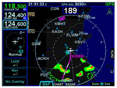
Decluttered Map with Onboard Weather Radar Overlay
