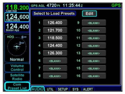
Preset frequencies can only be changed when the page is in edit mode. To put the page in edit mode using the touchscreen, touch the "Edit" box in the top right corner of the display. To put the page in edit mode using the right knob, move the cursor to the "Edit" box and press the knob button. The "Edit" box will appear in dark blue to indicate that the page is in edit mode.
