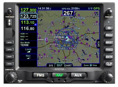
Supplemental IFD functions include a moving-map, flight management system (FMS), electronic charts, checklists, and a number of timer and calculator types of utilities. Optional IFD functions include control and display of remote transponders, weather radar, and external video. The system includes terrain alerting as well as an option for TAWS (or HTAWS).
