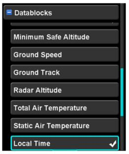
Once the datablocks category is expanded, the operation of the right knob is slightly different than the normal Setup Page operation. The outer knob selects the datablock "slot" to be affected. The inner knob selects the datablock that is to be displayed in the selected slot. The selected slot is shown with a blue background (except for the VLOC radio block). The selected datablock is shown with the typical cyan cursor surrounding the item.
