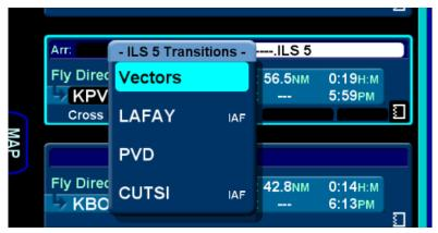
After having selected the procedure, including related transitions, the legs will be inserted into the flight plan and the corresponding destination airport field will contain the name of the procedure that was just inserted. In expanded view, a white bracket will be presented along the left side of the legs in the procedure, labeled with the name of the procedure.
