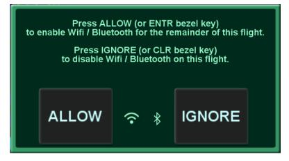
To disconnect WiFi and Bluetooth interfaces, either touch "Ignore" or press the CLR button. From that point on, the IFD will not connect with devices over those two interfaces.
