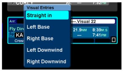
A visual approach consists of a single flight plan leg aligned with the runway heading terminating at the runway threshold. Altitude constraints cannot be entered on the visual approach leg. The area typically used to display altitude constraints is instead used to show the glideslope angle associated with the visual approach.
