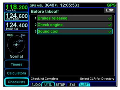
If a step inadvertently has been checked off as accomplished, it can be unchecked by selecting the step (touch it or use the bottom right knob) and then touching it a second time or pushing the knob to remove the checkmark. This will also toggle the "Checklist Complete" text back to "Checklist Not Completed".
