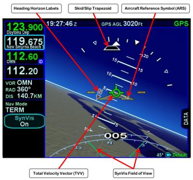
The SynVis field of view adjustment can be made by either pinch zoom gestures on the touchscreen display or by turning either of the bottom right knobs. Pushing the knob will restore the 45° field of view default value.
