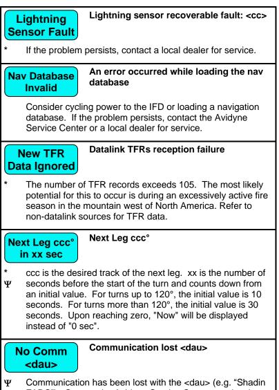
Y Communication has been lost with the <dau> (e.g. "Shadir FADC"). Contact the Avidyne Service Center or a local dealer for service.
