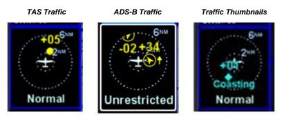
Traffic Advisories (TA) will generate a CAS message. Depending upon the type of traffic system installed, an aural alert may also be generated. Most installations will ensure the traffic system is in Standby or Ground mode on the ground and will automatically toggle to one of the enroute altitude modes per the table below.
