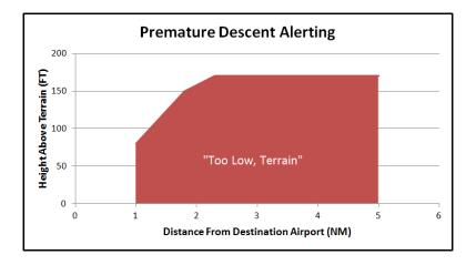
If a PDA alert has been triggered, a CAS message and aural alert "Too Low Terrain" will be issued and repeat every 6 seconds until it is acknowledged or the condition is no longer true. For the condition to no longer be true, the aircraft must clear the alerting altitude by 100 feet. So, for example, if the aircraft is 4 NM away from the airport and descended to 150 feet AGL, a climb to 270 feet AGL must be completed to clear the condition.
