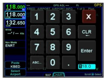
Each keyboard has a scratchpad in the lower right corner. The scratchpad is a free text field for data entry with some data entry validity logic applied to the data that is trying to be entered. For example, when trying to enter an invalid frequency, the IFD will
