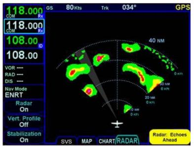
The "Stabilization" LSK is an on/off toggle of the radar's gyro stabilization.
