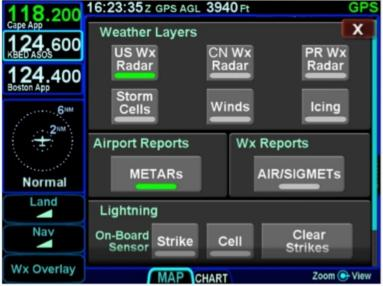
The options vary with the installed datalink device and subscription level.
