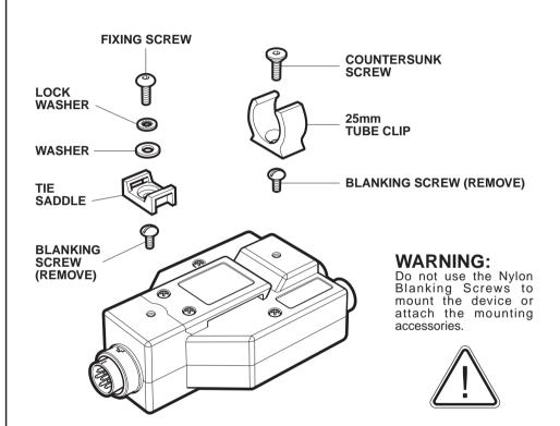
Depending on the application, small devices may be mounted permanently using Velcro, Screws, Tube Clips, or Cable Tie Saddles.
