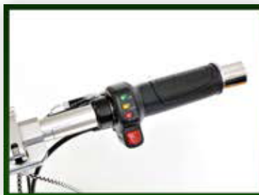
3 Power Modes: Pedal, Throttle, Pedal Assist
