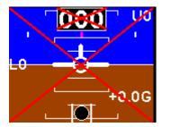
The display will have a red cross over the indicators to signal a SP-X sensor communication or sensor failure. Check the communication link between the AHRS-1 / MAG-1 and the SP-X sensors and that the SP-X sensors themselves are functional.
