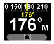
The F1 key pressed at a heading of 176 degrees. Currently the heading equals the course to steer as shown below the heading tape. No course steering indicators are shown.
