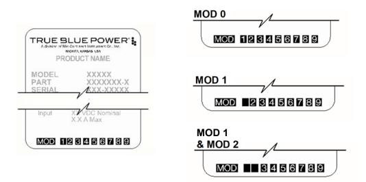
Figure 2.2.1 Nameplate and MOD Status Example
