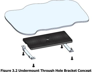
jure 3.2 Undermount Through Hole Bracket Conc (-1 Configuration Shown)
