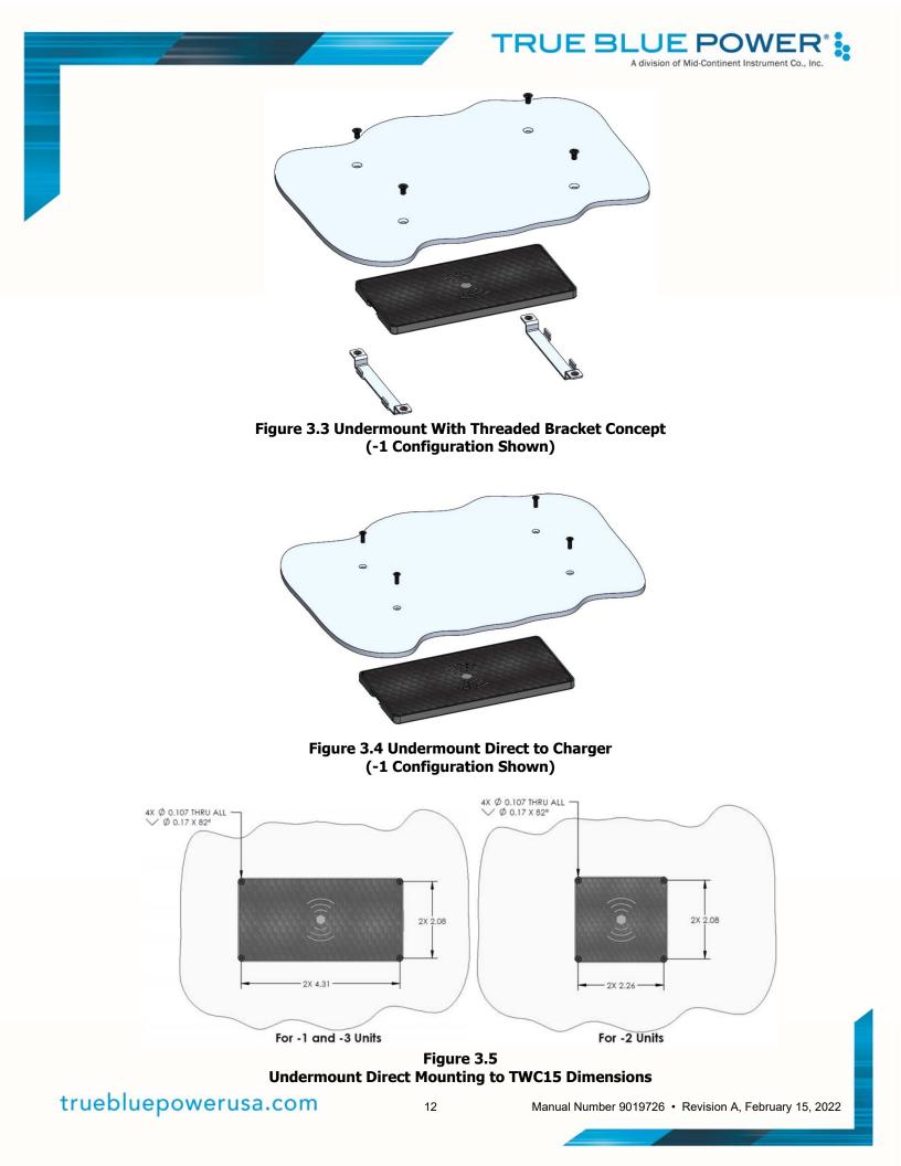
Mounting TWC15 units below the panel using a direct mount to the wireless charger requires countersinking holes (see Figure 3.5 above) for a #2 screw. Additionally, the label on top of the wireless charger has 4 small gray dots in each corner. A push pin can be used to punch through the label to allow the 2-56 screws (qty 4) to attach from above per Figure 3.6.
