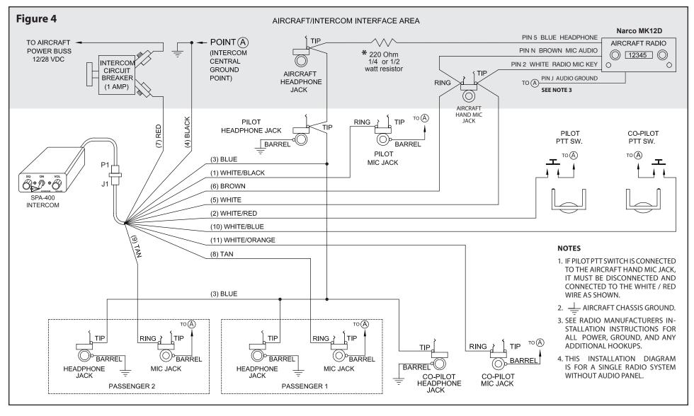
SPA-400 - Narco MK-12D Radio Installation Wiring Diagram
