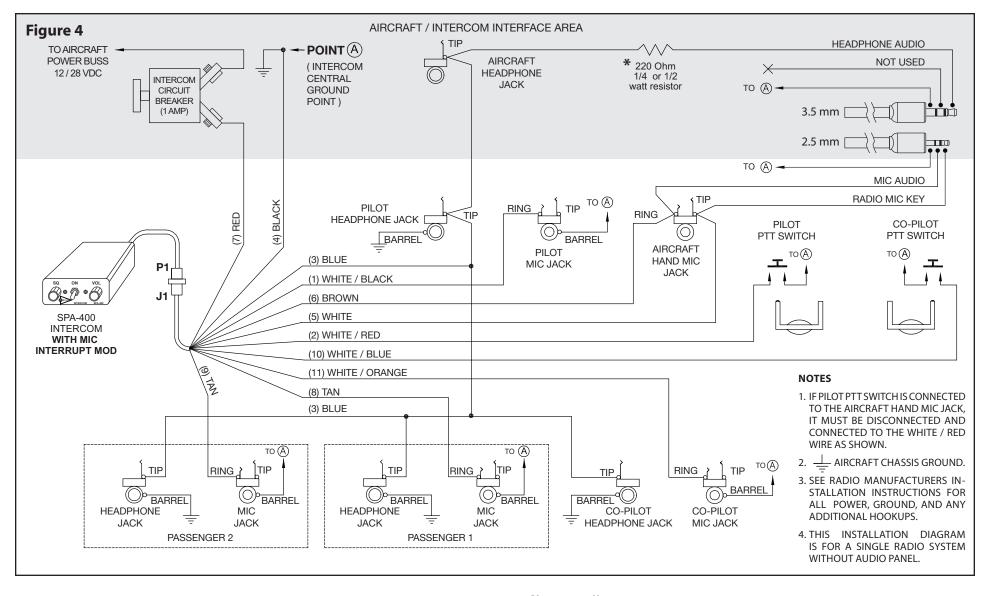
SPA-400 – ICOM A3, A6, A22, A24 Radio Installation Wiring Diagram
