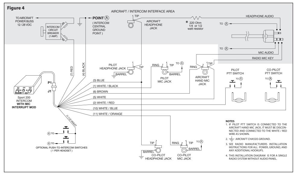
**Sport 200 – King KX99 Radio** Installation Wiring Diagram
