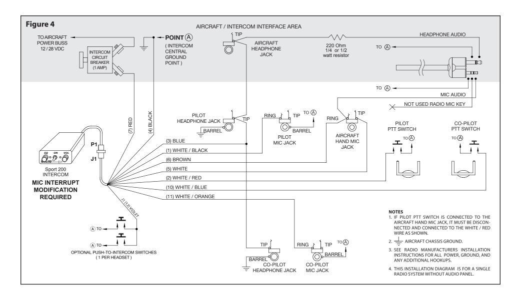
Sport 200 – ICOM A20, A21 Radio Installation Wiring Diagram
