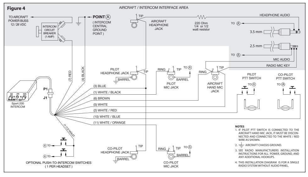
**Sport 200 – ICOM A4 Radio** Installation Wiring Diagram
