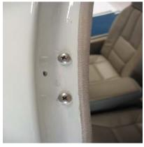
Install Sunvisor by placing mounting base through the screws and securing with washers and lock nuts provided. If desired, use silicone or other sealant like RTV around the heads of the #10 screws to seal from moisture.
