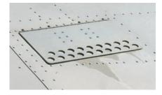
Figure 1-49 Speed brake.
