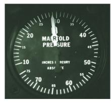
Figure 1-31 Manifold pressure gauge.
