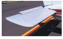
Figure 1-11 Stabilator with tab.
