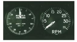
Figure 1-14 Manifold pressure gauge and tachometer.
