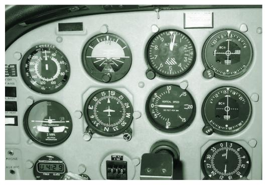
Figure 1-22 Typical instrument panel (Piper).
