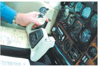
Figure 1-5 Traditional control wheel or yoke.
