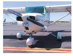
Figure 1-15 Tricycle landing gear.
