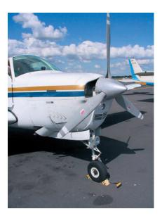
Figure 1-38 Constant speed propeller (Beechcraft Bonanza A36).
