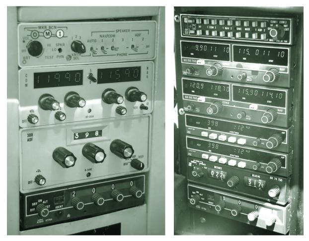
Figure 1-20 Radio control panels.
