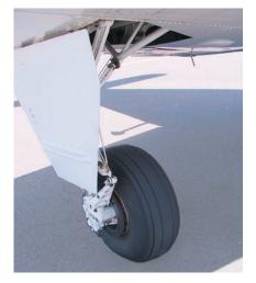
Figure 1-47 Retractable gear.
