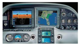
Figure 1-33 Cirrus instrument panel showing the primary flight display (PFD) and multi function display (MFD).
