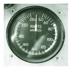
Figure 1-24 Airspeed indicator (ASI).
