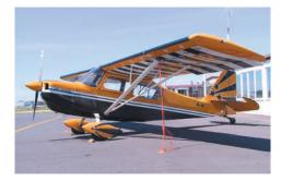
Figure 1-16 Tail wheel landing gear.
