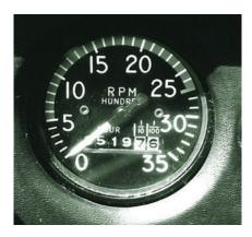
Figure 1-30 Tachometer.
