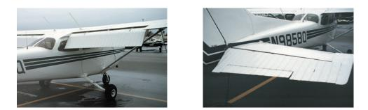
Figure 1-10 Flaps (left); elevator and trim tab (right).
