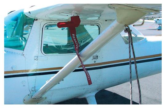
Figure 1-35 Pitot cover and tie-down rope.
