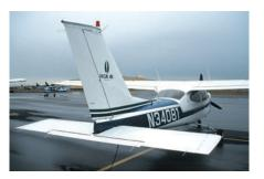
Figure 1-9 Left aileron (left); vertical stabilizer and rudder (right).
