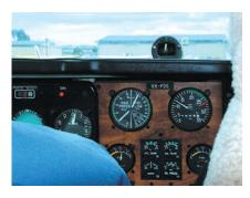
**Figure 1-39** Engine instruments—CSU.
