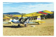
**Figure 1-42** Low-inertia tailwheel airplane.
