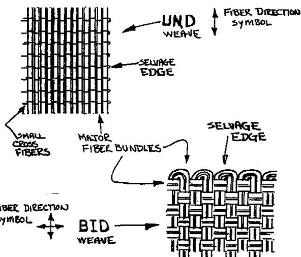
BID is generally used as pieces which are cut at a 45° angle to the selvage and laid into contours with very little effort. BID is often applied at 45° orientation to obtain a desired torsional or shear stiffness. UND is used in areas where the primary loads are in one direction and maximum efficiency is required, such as the wing skins and spar caps. Correct orientation of fibers is extremely important.
