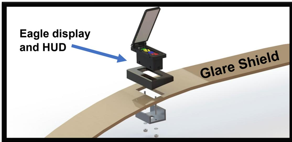
To accommodate the wide variety of aircraft, instrument panels, windshield slopes and mounting locations, Alpha Systems designed a mounting kit that replaces the standard plate and below dash angle brackets.
