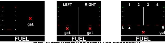
FUEL INSTRUMENT NOT INSTALLED CORRECTLY
