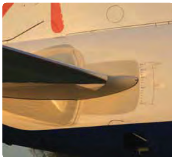
Figure 1-10. A stabilator and index marks on a transport category aircraft.
