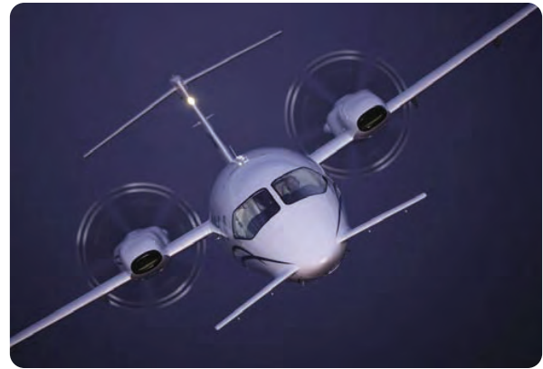
Figure 1-12. The Piaggio P180 includes a variable-sweep canard design, which provides longitudinal stability about the lateral axis.
