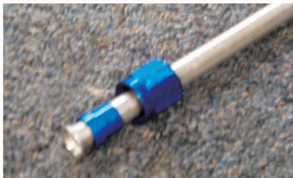
Flared tube assembled with sleeve and nut.
