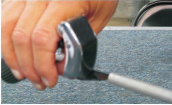
Deburring inside of edge.
