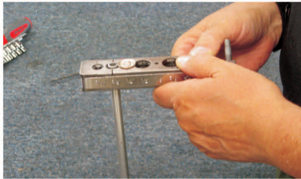
Setting tube in die (dime's thickness over top).
