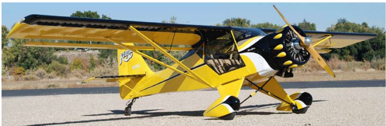
The Kitfox has been a very popular design that is sold as a complete kit, with engine, and has folding wings.
