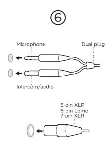
Insert the aircraft connector into the aircraft control panel.
