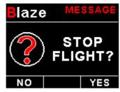
Press the F1/Up button during the normal display mode to manually start/stop a flight. This key is only active if the MAP-4 is setup to select the manual flight option under the "TIMERS" setup menu.
