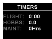
This display can be accessed by rotating the rotary control during the normal display mode. The flight, Hobbs and Maintenance Timers are shown.
