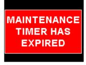
This function allows you to set an engine maintenance timer. This timer is set in engine hours and it will count down to zero when the engine RPM is greater then the "HOBBS RPM". A good use for this function is to set the hours until your next spark plug change or engine inspection. Use the rotary control to change the value.
