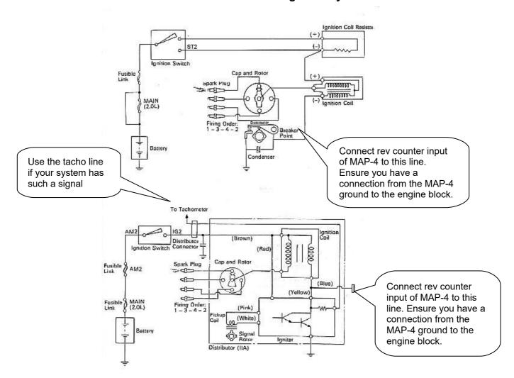
Electronic ignition system with conventional ignition coil
