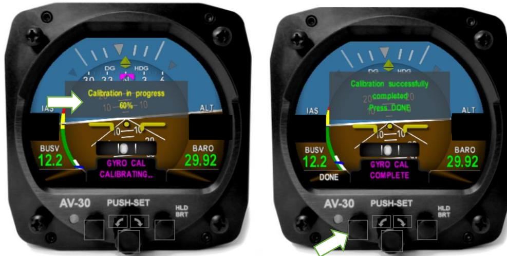
Figure 31 - Gyro Calibration Procedure
