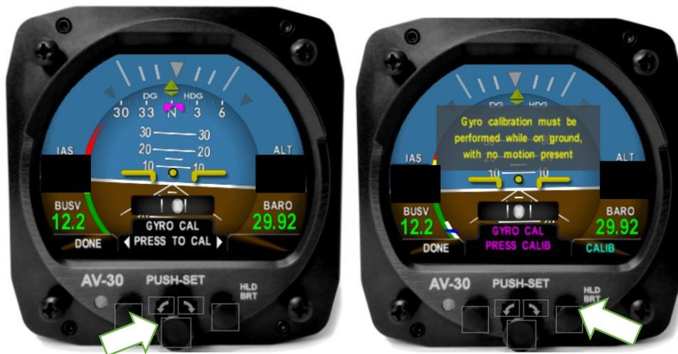
Figure 30 - Gyro Calibration Selection
