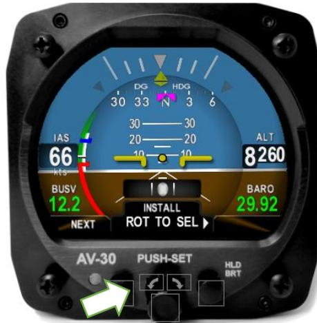
Figure 29 - Install Mode Selection
