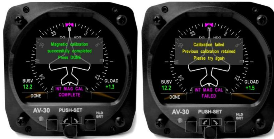
Figure 34 - INT MAG CAL Success and Failure Screens
