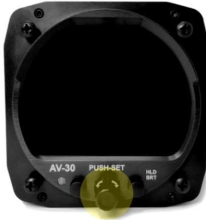
*Figure 22 – Installation Menu Access*
