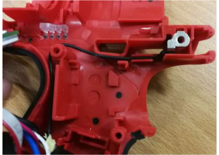
STEP 2: Assemble HV terminal over screw boss and route HV terminal wire through channels and traps as shown.
