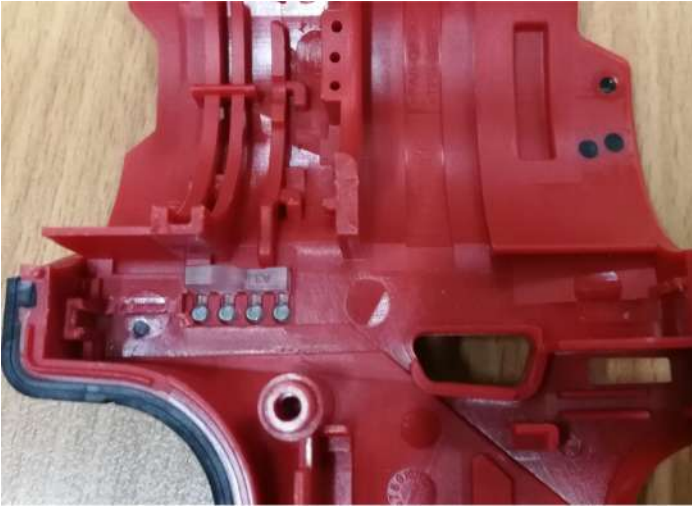
STEP 1: Insert light pipe in cavity of left housing half-support.
