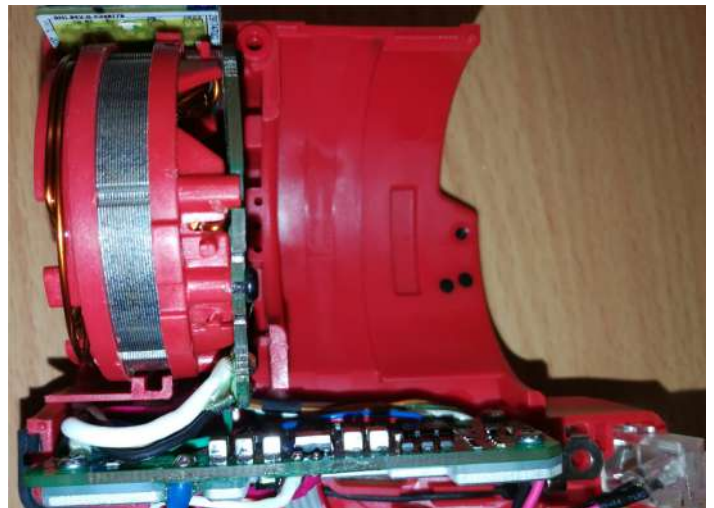
STEP 6: Assemble stator over pop switch wires. Be sure stator is seated firmly and squarely in housing half.
