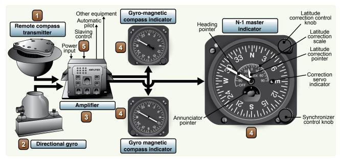
Figure 3-8. N-1 compass system components.
