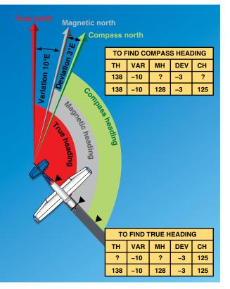
Figure 3-5. *Find true heading by working backwards.*
