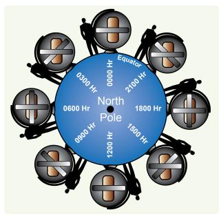
Figure 3-10. Apparent precession.
