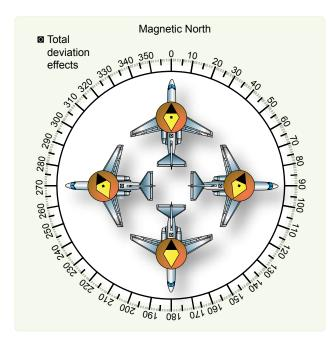
Figure 3-6. Deviation changes with heading.
