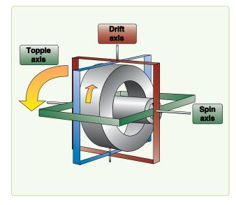
Figure 3-9. Gyroscope axes.
