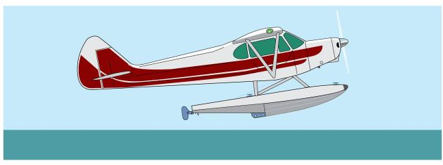
Figure 6-2. The touchdown attitude for most seaplanes is almost the same as for taxiing on the step.
