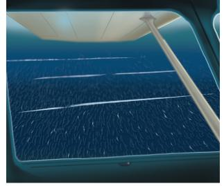
Figure 6-1. Wind streaks show wind direction accurately, but the pilot must determine which end of the streak is upwind.
