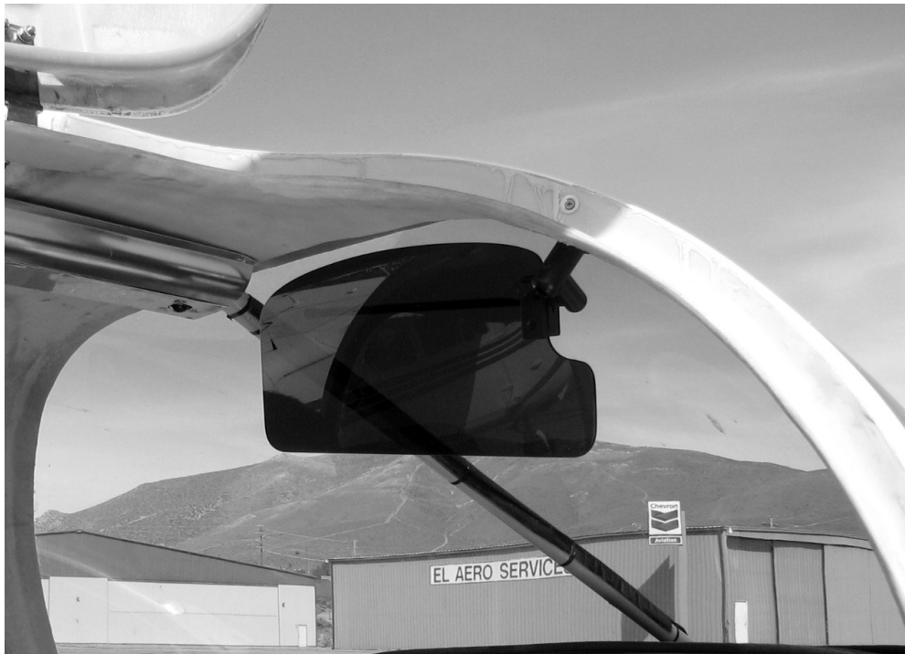
Co-Pilot Visor Installed
