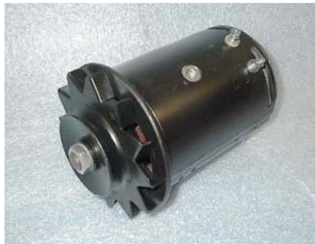
Figure 3-13 Belt Driven Generator.
