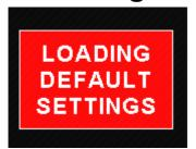
Press and hold the F1/Up button and rotary control during power up to load the preprogrammed factory default settings. The following screen will be displayed:
