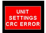
Unit settings CRC error. Load default settings to restore to factory defaults. If the error message still persists then it could possibly be a non-volatile memory failure in which case the instrument will then have to be returned to the factory.
