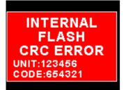
Internal flash CRC error. The instrument does a firmware check on the program when power is applied to the instrument. If the program is corrupt in any way then the internal flash CRC error will be displayed. Reload the instruments firmware and load default settings. If the error message still persists then it could possibly be an internal flash memory failure in which case the instrument will then have to be returned to the factory.
