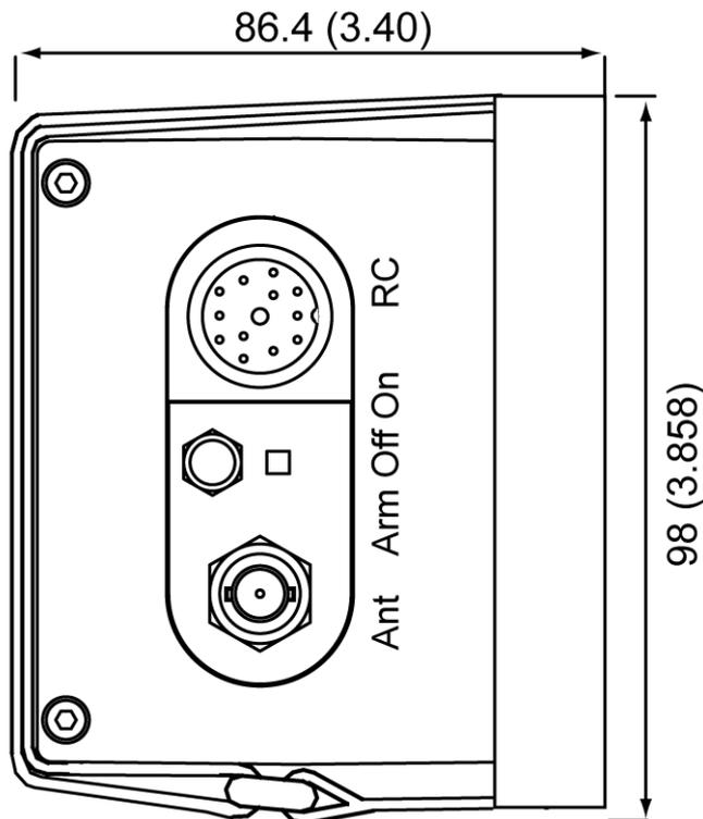
*Figure 36: Outline dimensions and weight with Compact Universal Mounting Bracket P/N S1840502-02*
