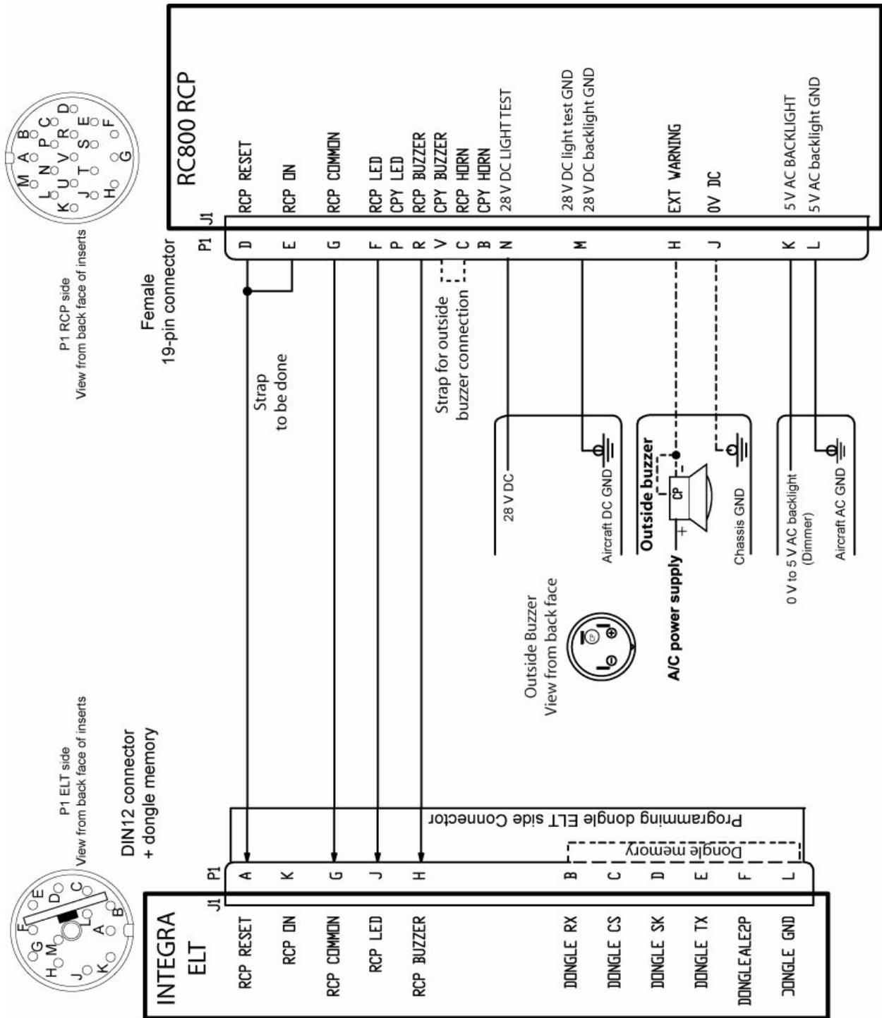
Figure 64: RC800 Wiring Diagram with Dongle INTEGRA / SA
