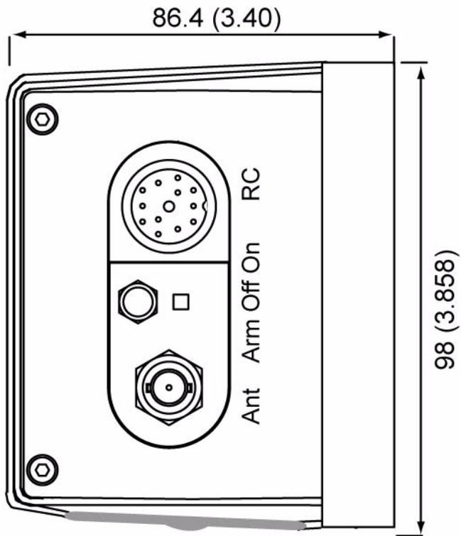
*Figure 39: Compact Mounting bracket P/N S1840502-01, Outline dimensions and weight*
