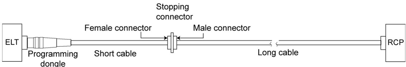
NOTE 2: The mounting of a stopping connector may be skipped by using our pre-wired Programming Dongle ASSY (P/N S1820514-06). This dongle is fitted with the Programming Dongle (S1820514-01) on the ELT side and a female DIN-12 connector on the RCP side. In this case, a RCP bundle must be fabricated using a male DIN-12 connector (reference P/N S1820514-03 or BINDER 680-1-09-0329-00-12) and the relevant mating connector of the RCP.
