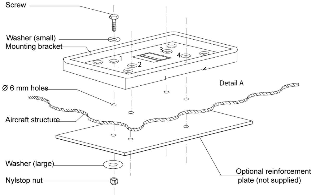
**D. ELT installation procedure***(1) Installation with hook-and-loop mounting brackets*
