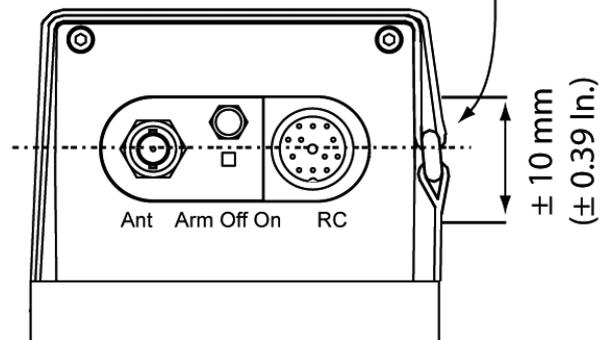
(2) *ELT Installation with draw latch mounting bracket P/N S1850551-02*
