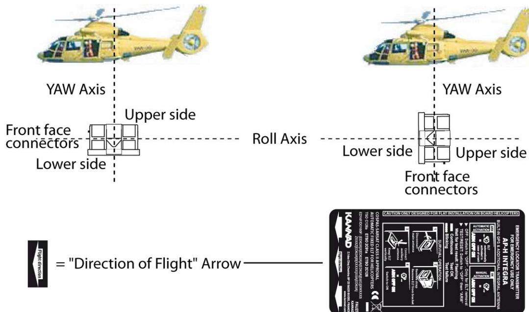
The "Direction of Flight " arrow shall point towards the front or the bottom of the helicopter (and not pointing  $45^\circ$  downwards):
