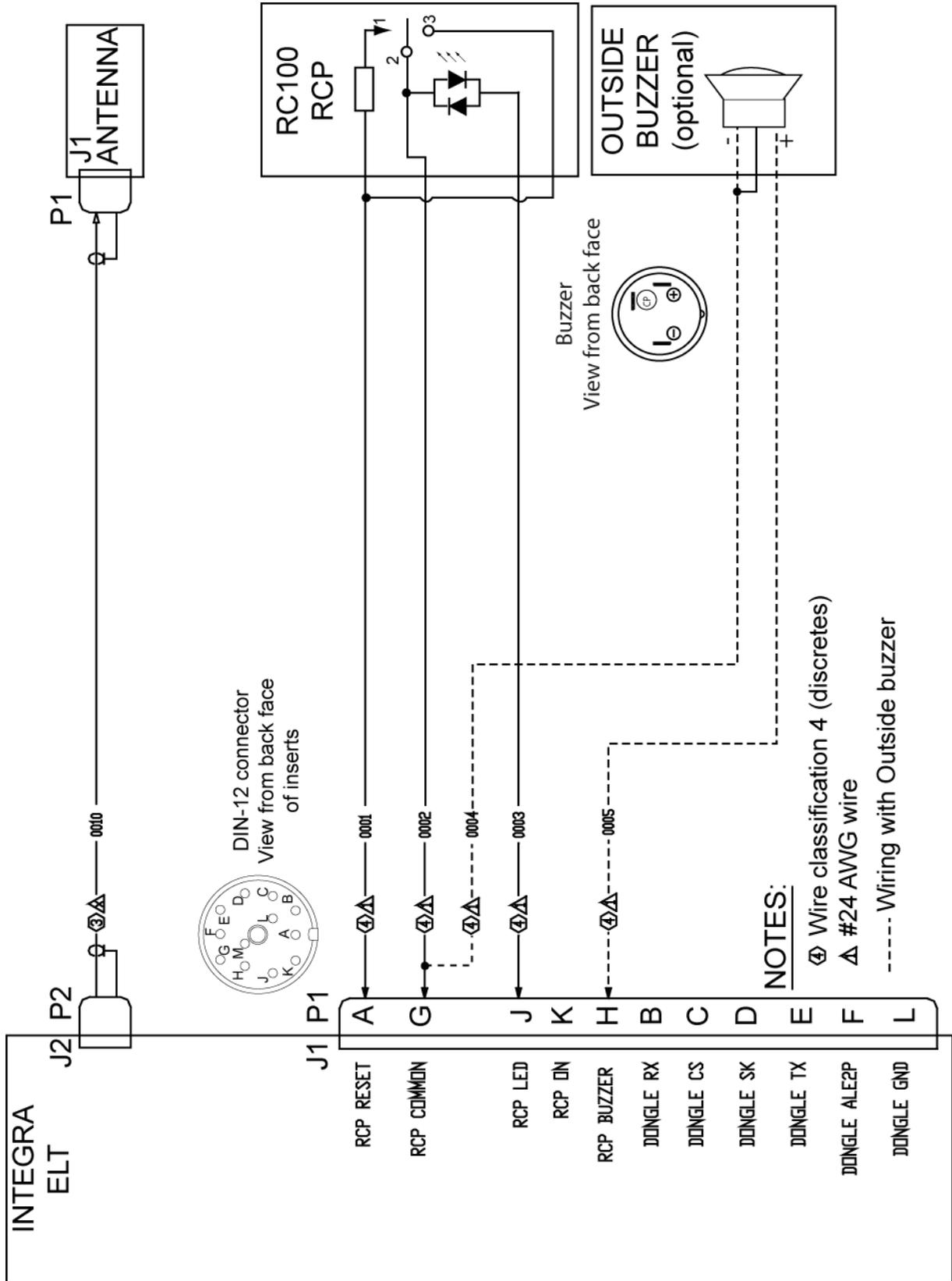
Figure 58: RC102 Wiring diagram
