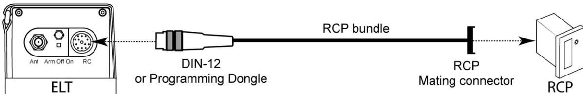
NOTE 1: in order to easily remove the programming dongle, when the RCP is connected to the ELT via a Programming Dongle (P/N S1820514-01), it is recommended to fit its cable with a stopping connector as close as possible to it (see figure below).
