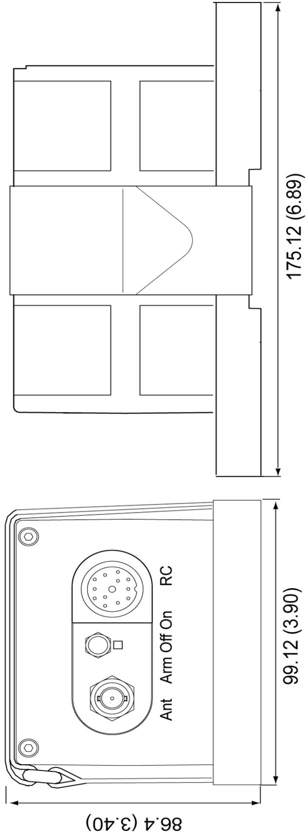
Figure 37: Outline dimensions and weight with Bracket Universal for INTEGRA ARINC e-NAV for ELT (AF), P/N S1850551-02
