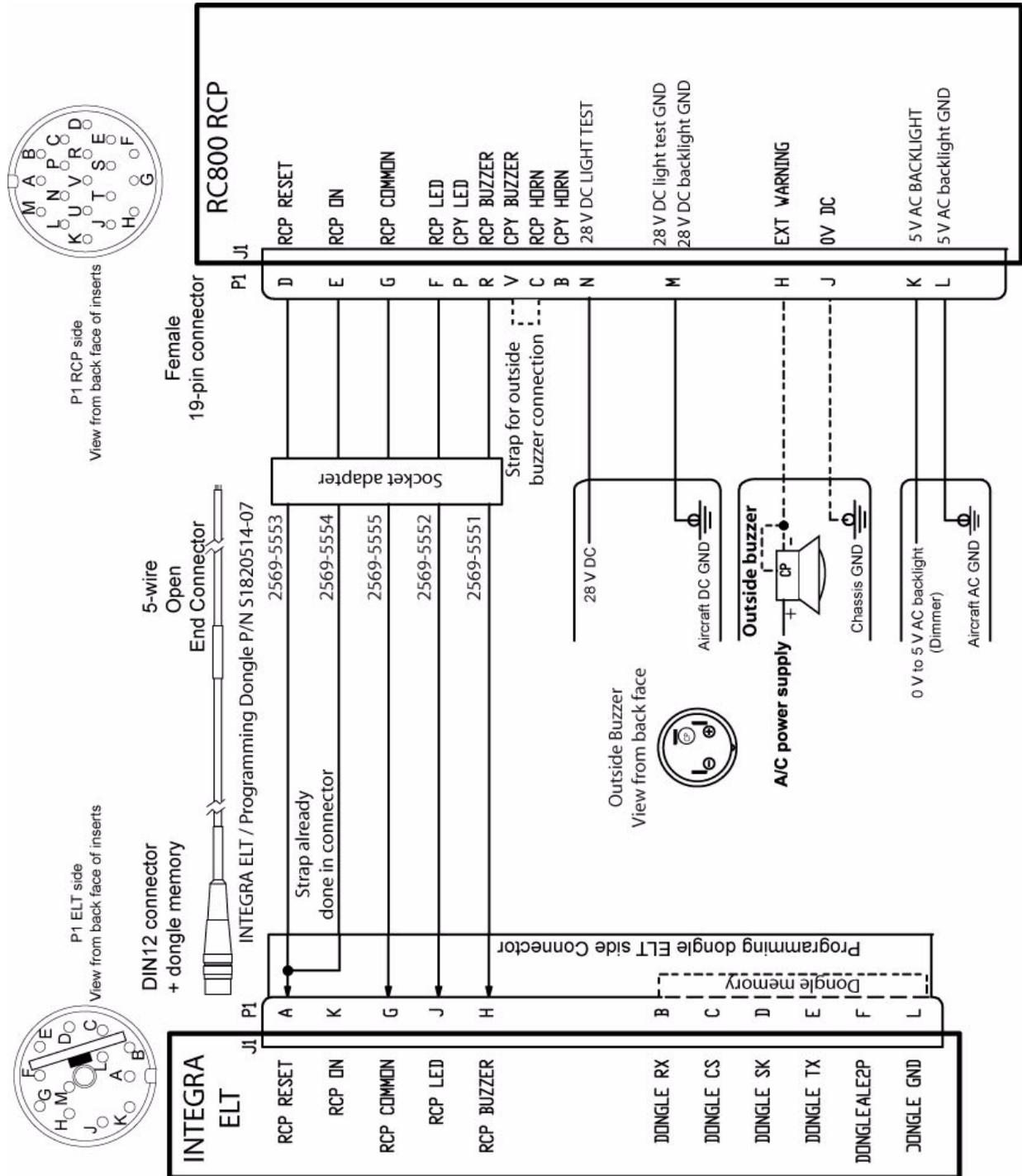
Figure 66: RC810 Wiring Diagram with standard connector / dongle
