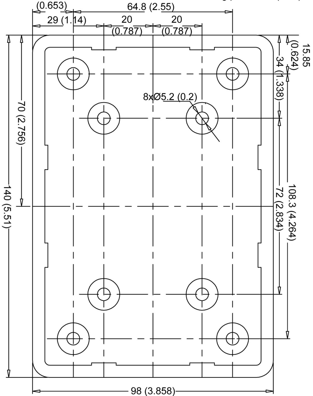
*Figure 40: Compact Universal Mounting bracket P/N S1840502-02, Outline dimensions and weight*
