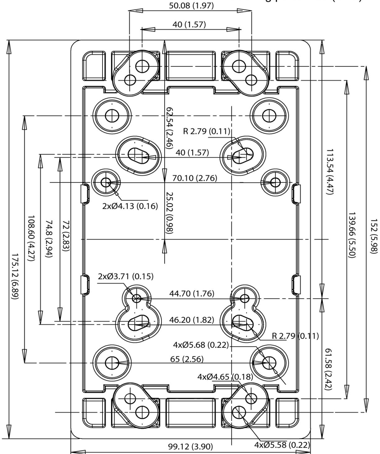
*Figure 41: Bracket Universal for INTEGRA ARINC e-NAV for ELT (AF)
