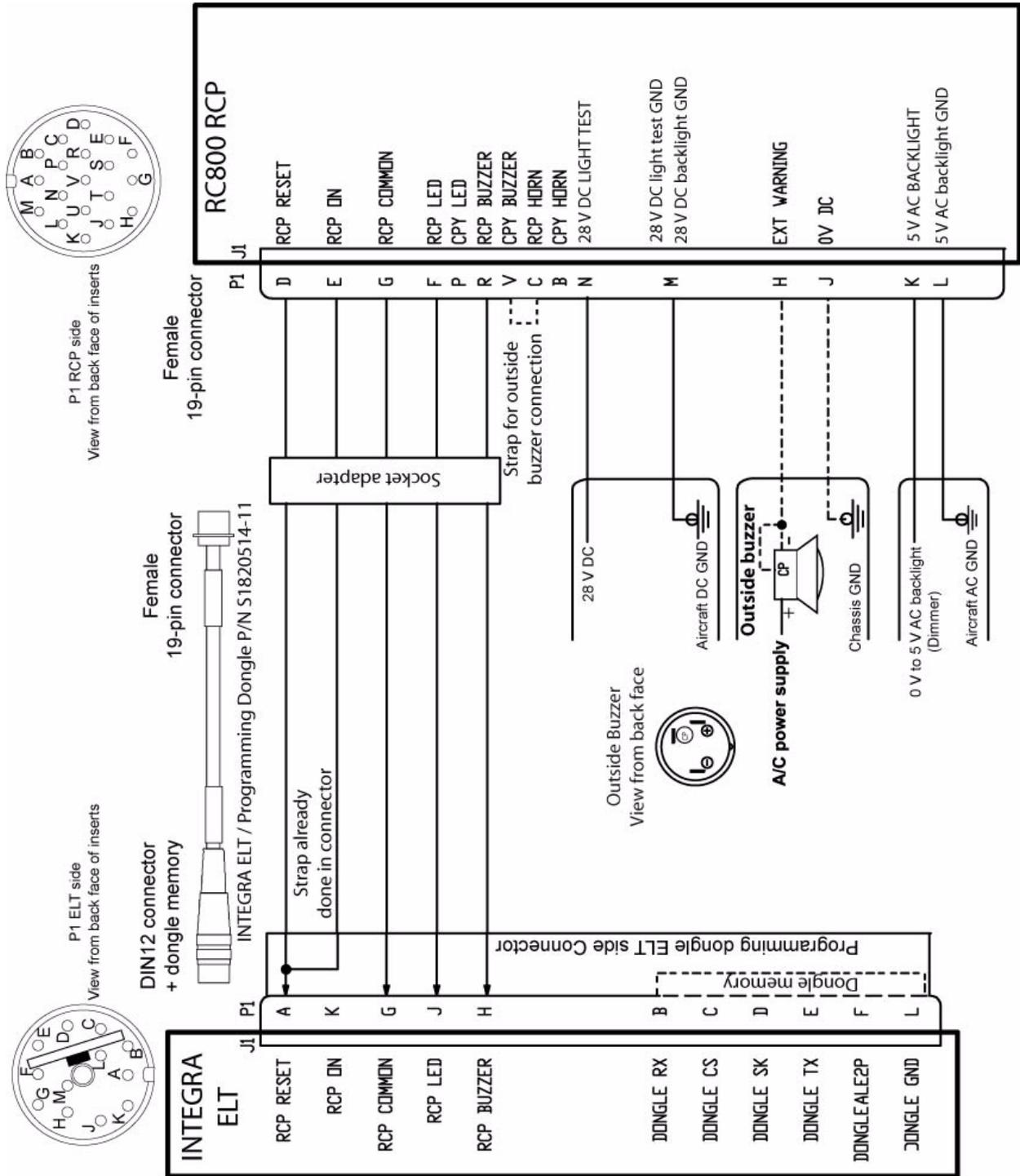
Figure 65: RC800 Wiring Diagram with Dongle INTEGRA / LR
