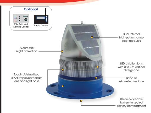
The solar powered AV-70 is a field proven aviation light that offers enormous benefits over traditional battery and hard-wired aviation lights including low maintenance and no underground wiring.
